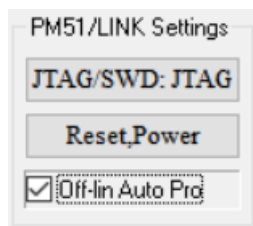
Figure 4.6-1 setting of offline burning. When the chip is connected with the burner, it will be automatically burned. There is no need to press the key, so it is easy to operate. If there is a large capacitance on the board, please adjust the power down time / reset level duration (MS) according to figure 4.5-2
