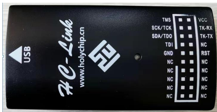
Figure 2-2 hc-link V3.0 (tk-rx is the RX of hc-link, tk-tx is the TX of hc-link)
