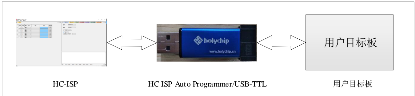
Figure 2-1 hardware connection (HC ISP auto programmer)
